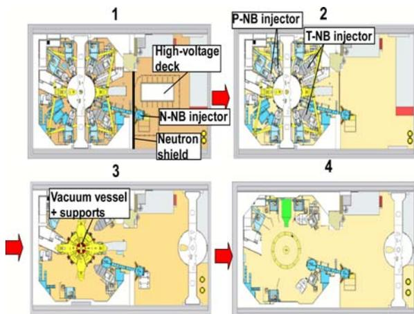
Fig.1 Sequence of disassembly in JT-60U. 1) Original layout, 2) Removal of HV deck and neutron shield wall, 3) Removal of P-NB tanks, 4) Removal of vacuum vessel
