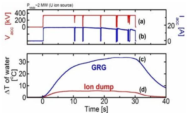
Fig.4 Time evolutions of the beam energy (a), the beam current (b), water temperature rise on the grounded grid (c), water temperature of the ion dump (d)
