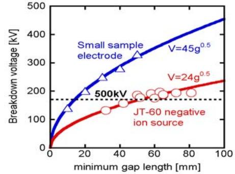
Fig.6 Vacuum insulation in a gap between the grids in the JT-60negative ion source
