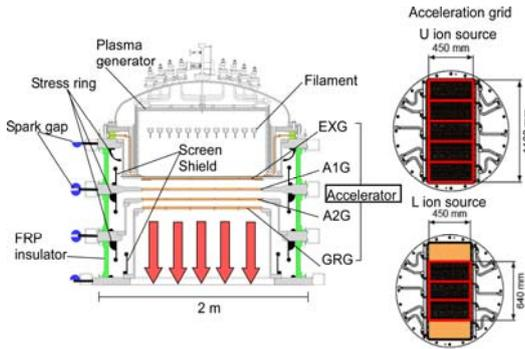
Fig.5 Schematic diagram of the original JT-60 negative ion source
