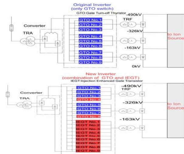
Fig.2 Inverters in the acceleration power supplies on JT-60U (upper) and JT-60SA(lower)
