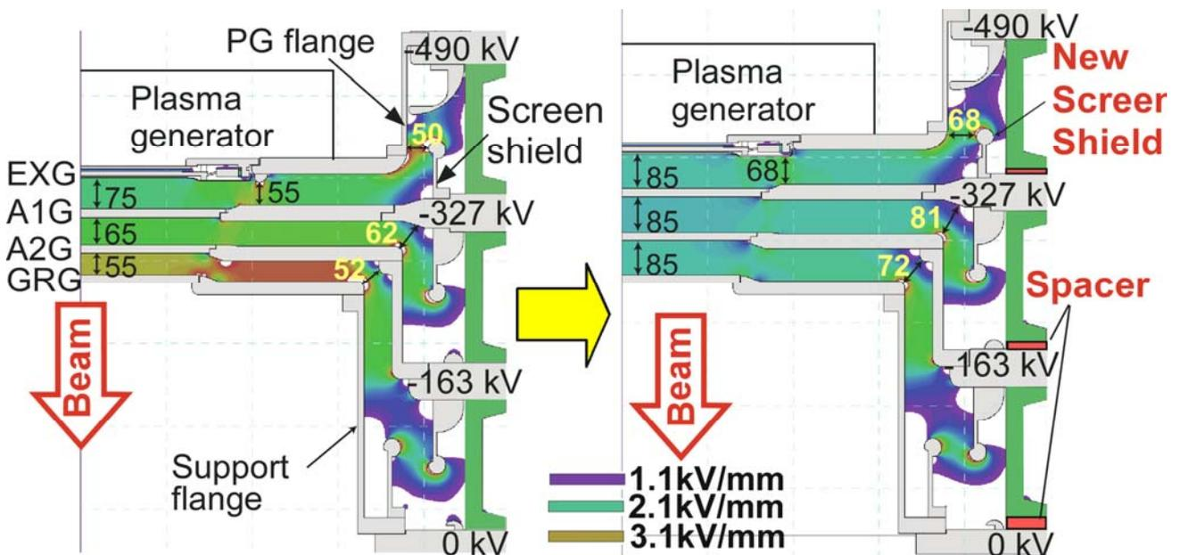
Fig.7 Contour maps of electric field strengths at 500 kV in the original (left) and the modified (right) ion sources.
