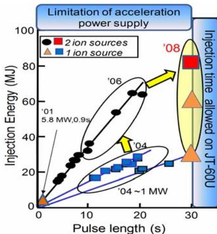
Fig.3 Progress in the long pulse injection on JT-60U. The ion extraction areas of the two ion sources (the U and L ion sources) are different each other (see Fig.5), so that the injection powers from two ion sources are different.
