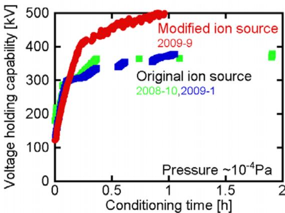
Fig.8 Voltage holding capabilities without beam acceleration for the original and the modified ion sources
