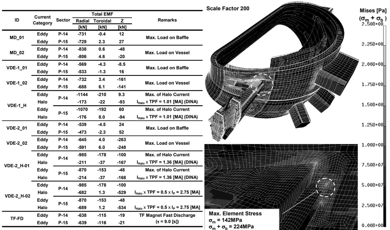
Fig.3 EM force analyses results (left), and the structural analysis result of the VDE-2 static stress distribution (right). Higher stress intensity region are observed around the stem joint to the outerwall.
