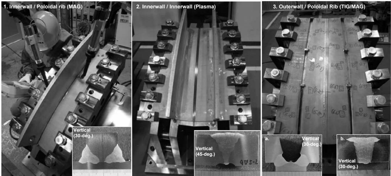
Fig.4 Middle Size Test Manufacture (at the Outboard R1420). 1. Twin MAG fillet welding; its length unwelded and position dependences are surveyed. 2. Plasma welding; the key-hole weldment as a first layer, and the TIG-like filled as the others. 3. TIG welding as a first layer full penetration (a.) and MAG continuous plug welding (b.).
