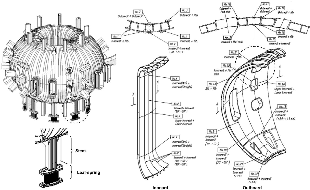
Fig.1 JT-60SA Vacuum Vessel and the gravity support (left), 40 toroidal degree (two sectors) of the inboard (middle) and the outboard with port bores (right) are exhibited with various types of weldments. The region circled in the outboard is the R1420 corresponding to the medium size test manufacture.
