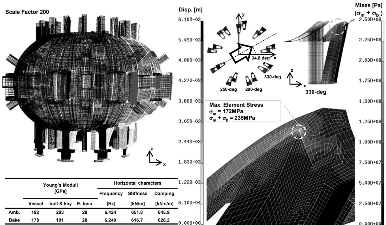
Fig.2 Response spectrum analysis of the seismic event. Maximum displacement responses and dynamic characters of the VV corresponding to each state (left), and element stress plot at the joint between the stem and the VV bottom (right). DRS is input in the weakest direction; 34.8 deg., as explained by the lowest natural frequency.
