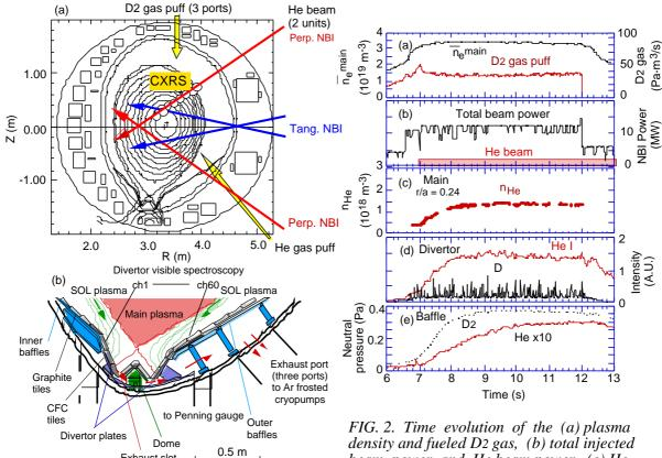
FIG. 1. (a) The cross section of an ELMy Hmode plasma in He exhaust experiments. The directions of He-NBI and heating NBI, the locations of He and D2 gas puff, and the viewing position of CXRS for the He density measurement are shown. (b) The structure of W-shaped pumped divertor of JT-60U after the divertor modification.
