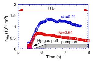
FIG. 7. Comparison of the time evolution of the He density at r/a = 0.21 inside the ITB and r/a = 0.64 outside the ITB in a reversed shear plasma ( $I_P = 1.7$  MA,  $B_t = 3.73$  T, vol.= 65 m<sup>3</sup>,  $P_{NB} = 6$  MW, deuterium) with He pumping.
