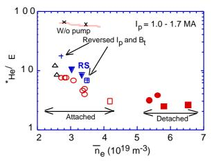
FIG. 4. The ratio of  $\tau^*_{He}/\tau_E$  confinement time of helium as a function of the lineaveraged electron density in the main plasma in various operation modes (attached and detached divertor, reversed  $I_P$  and  $B_t$ , with and without He pumping).
