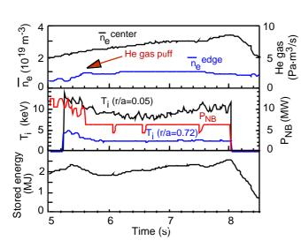
FIG. 5. Time evolution of a typical reversed shear discharge ( $I_P = 1.7 \text{ MA}, B_t = 3.73 \text{ T},$ vol. = 65 m<sup>3</sup>,  $P_{NB} = 6 \text{ MW}$ ) with He pumping.
