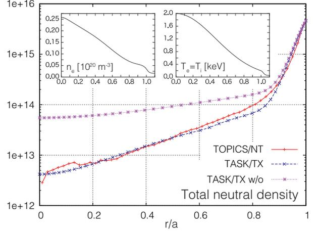
Fig. 4 Comparison of the neutral density profiles calculated by TOPICS/NT, TASK/TX and that without any special treatment for the thermal neutral transport modeling in a quasi-steady state at  $t = 0.5$  s, in the lower plasma density case.
