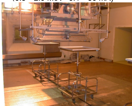
Electron irradiation room with conveyor system
