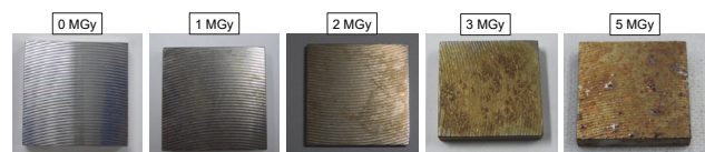
Fig. 2. The surface of nickel coated sample after irradiation.
