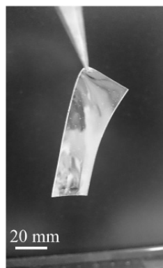
Fig. 1 An example of self-supported PDMS thin film prepared by spin-coat process for PBW procedure. MZ waveguide was formed inside of this PDMS film by 750 keV proton microbeam.
