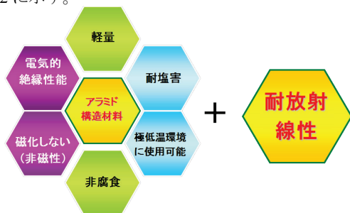
Fig. 2 Performance of new braided aramid fiber bar.
