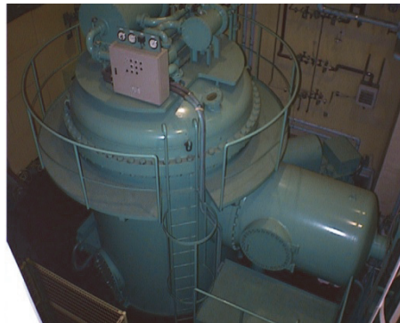
Electron accelerator (0.5~2.0 MeV 0.1~30 mA)
