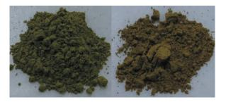
Fig. 1 Nickel ferrocyanide prepared (right; after Cs adsorption).
