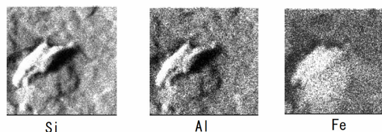
Fig. 1 Two-dimensional elemental mappings of Si, Al and Fe for Fe(III)-bentonite sample.
