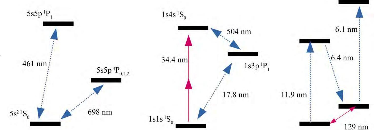
a) level scheme in Sr at visible wavelengths, used for state-of-theart atomic lattice clocks
