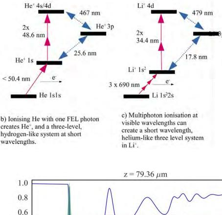
Coherent two-photon excitation can lead to yoked superfluorescence, where two cascade decays are inter-dependent. This is a potential route to creating superfluorescenece at shorter wavelengths than the incident radiation.
