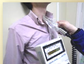
applied NaI(Tl) scintillation survey meter as substitution
