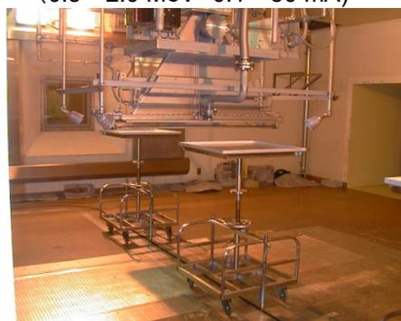
Electron irradiation room with conveyor system
