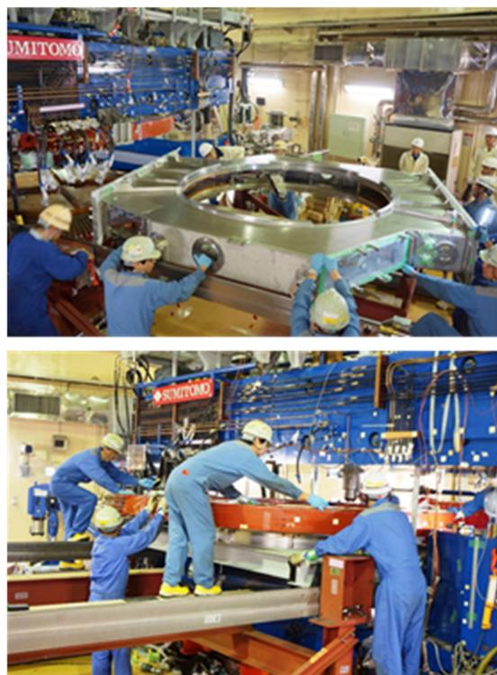
Fig. 2. Pictures of the main coil replacement work. Removing the vacuum chamber (upper) and the upper main coil (lower) from the magnet yoke.
