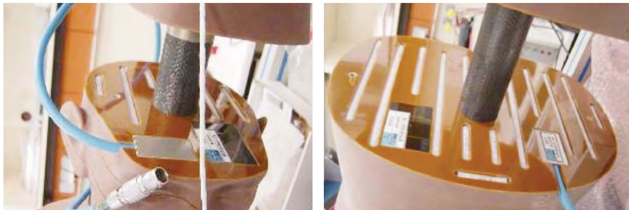
Fig. 3A: View of the head (left) and lower part of the torso (right) of MATROSHKA with the integrated passive and active radiation detectors. Passive detectors are integrated in polyethylene tubes and in the "organ dose" packages. The sensor for the active Silicon-Scintillator Device (SSD) is shown with the blue cable connecting to the base structure. The white cable connects to a temperature sensor in the head of the phantom. The pictures were taken during detector integration at DLR prior to the launch of the facility.
