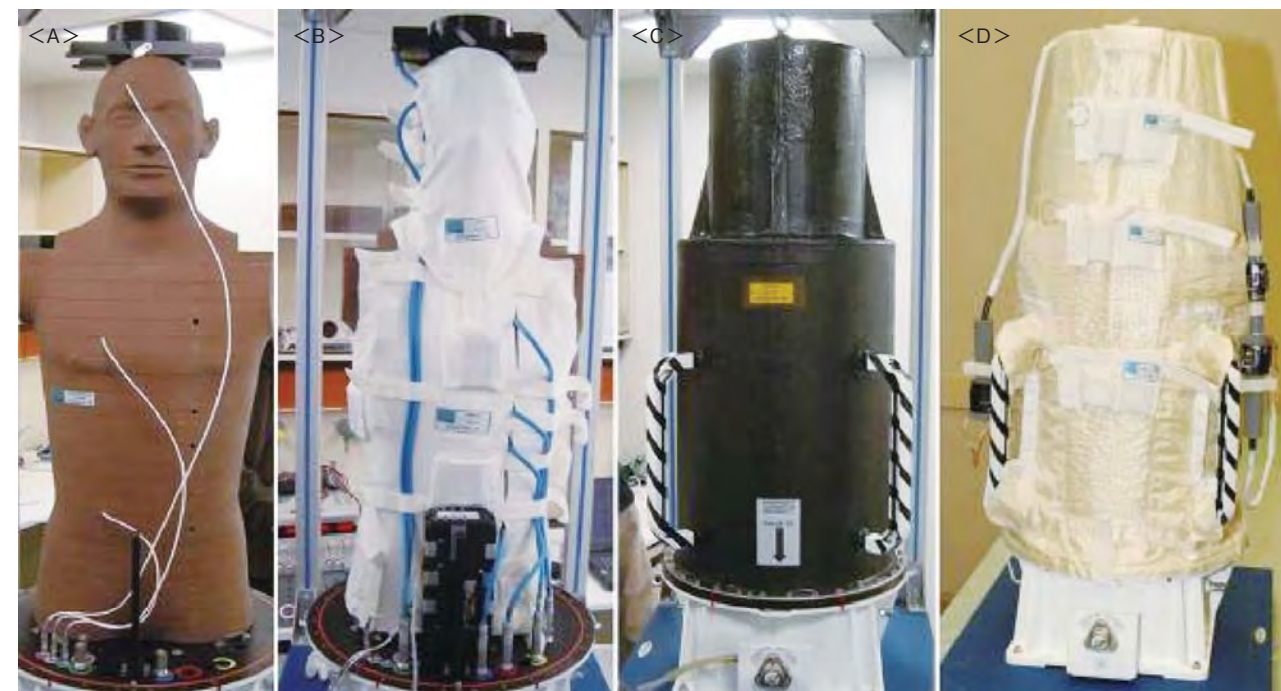
Fig. 2: The MATROSHKA phantom from left to right: <A> anthropomorphic upper torso equipped with and active detector systems, <B> torso with poncho and hood equipped with passive detector systems for skin dose measurements, <C> carbon fibre container to simulate the astronaut's space suit, <D> facility close to launch equipped with multi layer insulation (MLI) for thermal protection
