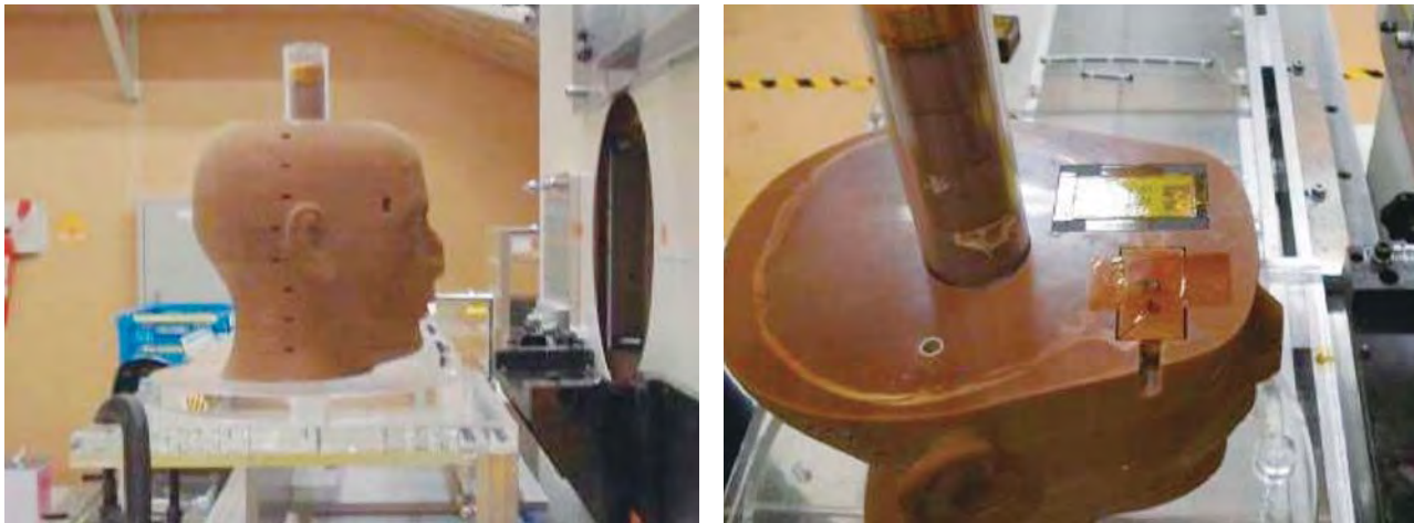
Fig.12:<Left> Phantom head equipped with TLDs in the Biology Room at NIRS; <right> TLD and CR-39 detectors in "Eye organ dose box" in Slice #3 of the phantom
