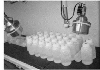
Figure 5.3: Bottle phantom (70-kg-configuration) in the WBC.
