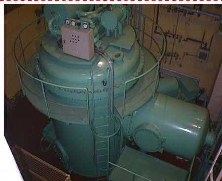
Electron accelerator (0.5~2.0 MeV, 0.1~30 mA)
