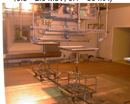
Electron irradiation room with conveyor system
