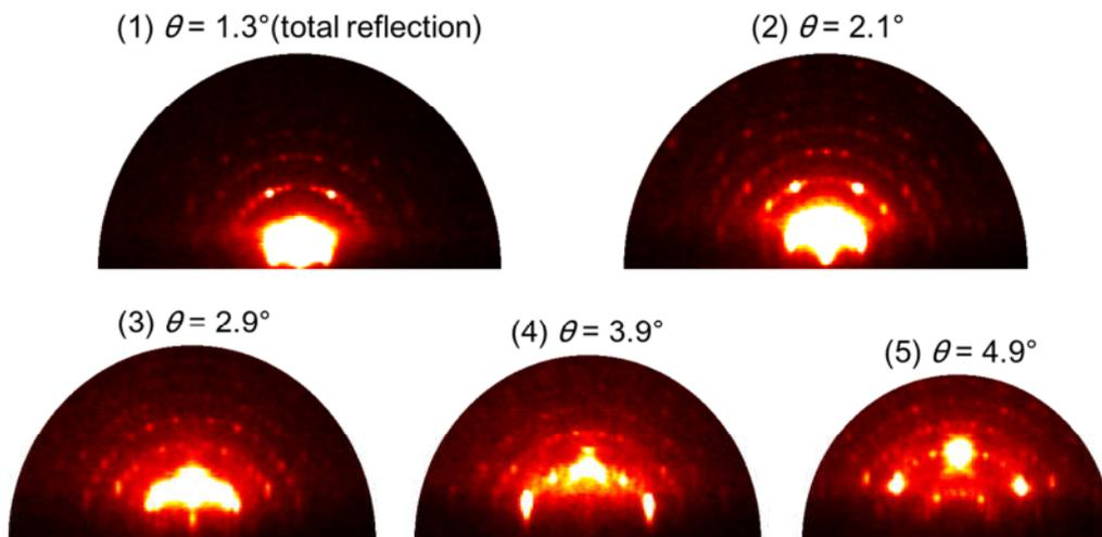
Figure 1. RHEPD patterns observed with a brightness-enhanced high-intensity positron beam.
