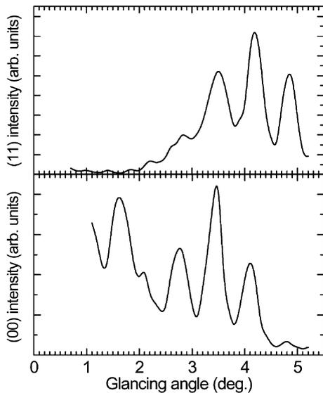
Fig. 4. Rocking curves of the (00) and (11) spot from Si(111) surface treated with  $\text{NH}_4\text{F}$  solution for the  $[11\bar{2}]$  incidence.
