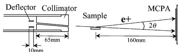
Fig. 1. Schematic drawing of the RHEPD experimental setup.
