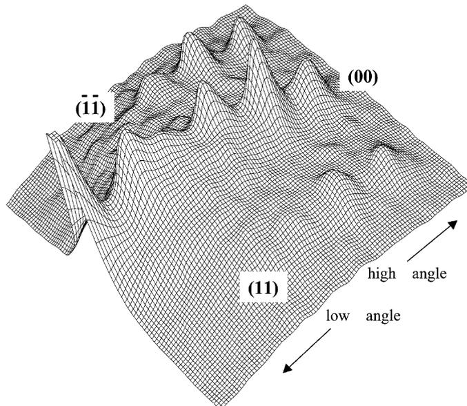
Fig. 3. A continuous photography of the zeroth Laue zone from Si(1 1 1) surface treated with  $\text{NH}_4\text{F}$  solution for the  $[1\ 1\ \bar{2}]$  incidence at  $\theta = 0.5\text{--}5^\circ$ .
