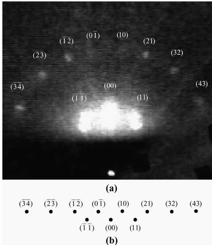
Fig. 2. (a) RHEPD pattern from Si(1 1 1) surface treated with  $\text{NH}_4\text{F}$  solution for the  $[1\ 1\ \bar{2}]$  incidence at glancing angle of  $4.0^\circ$ . (b) Reciprocal lattice of bulk truncated Si(1 1 1) surface which corresponds to diffraction indices shown in Fig. 1(a).
