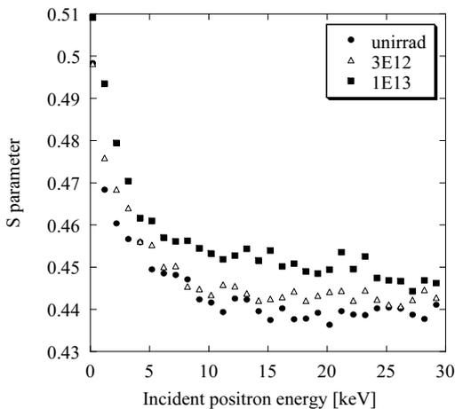
**Fig. 1** S-parameter for unirradiated and irradiated Fe-50 at.%Rh alloys as a function of incident positron energy.
