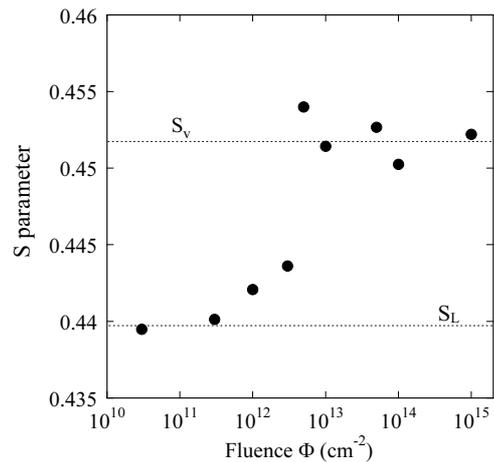
**Fig. 2** Change in average S-parameter as a function of  $^{136}\text{Xe}$  ion-fluence.
