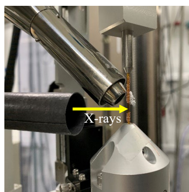
Figure 1. Photograph of the sample capillary wrapped with a copper wire at low temperature.
