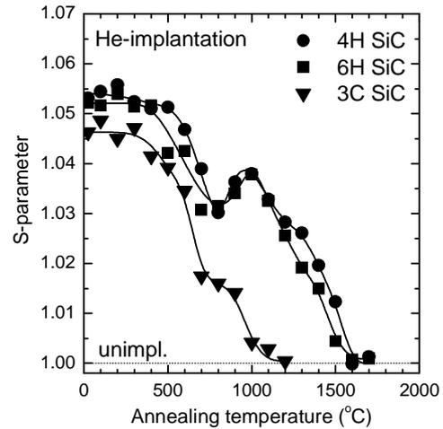
Fig. 2 Annealing behavior of normalized  $S$ -parameter for  $n$ -type 3C, 4H and 6H SiC epilayers after multiple He-implantation.
