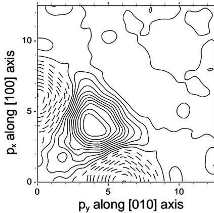
Fig. 3 ACAR spectrum from silicon vacancies in 3C SiC after 1MeV electron irradiation to a dose of  $6 \times 10^{17}$  e<sup>-</sup>/cm<sup>2</sup>. Solid and broken lines represent positive and negative values, respectively. Counter spacing is 10% to the maximum.
