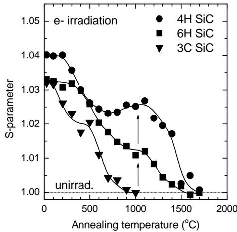
Fig. 1 Annealing behavior of normalized  $S$ -parameter for  $n$ -type 3C, 4H and 6H SiC epilayers after 2MeV electron irradiation to a dose of  $3 \times 10^{17} \text{ e}^-/\text{cm}^2$ .
