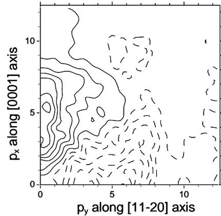
Fig. 4 ACAR spectrum from silicon vacancy related defects in 6H SiC after 2MeV electron irradiation to a dose of  $3 \times 10^{17}$  e<sup>-</sup>/cm<sup>2</sup>. Solid and broken lines represent positive and negative values, respectively. Counter spacing is 5% to the maximum.
