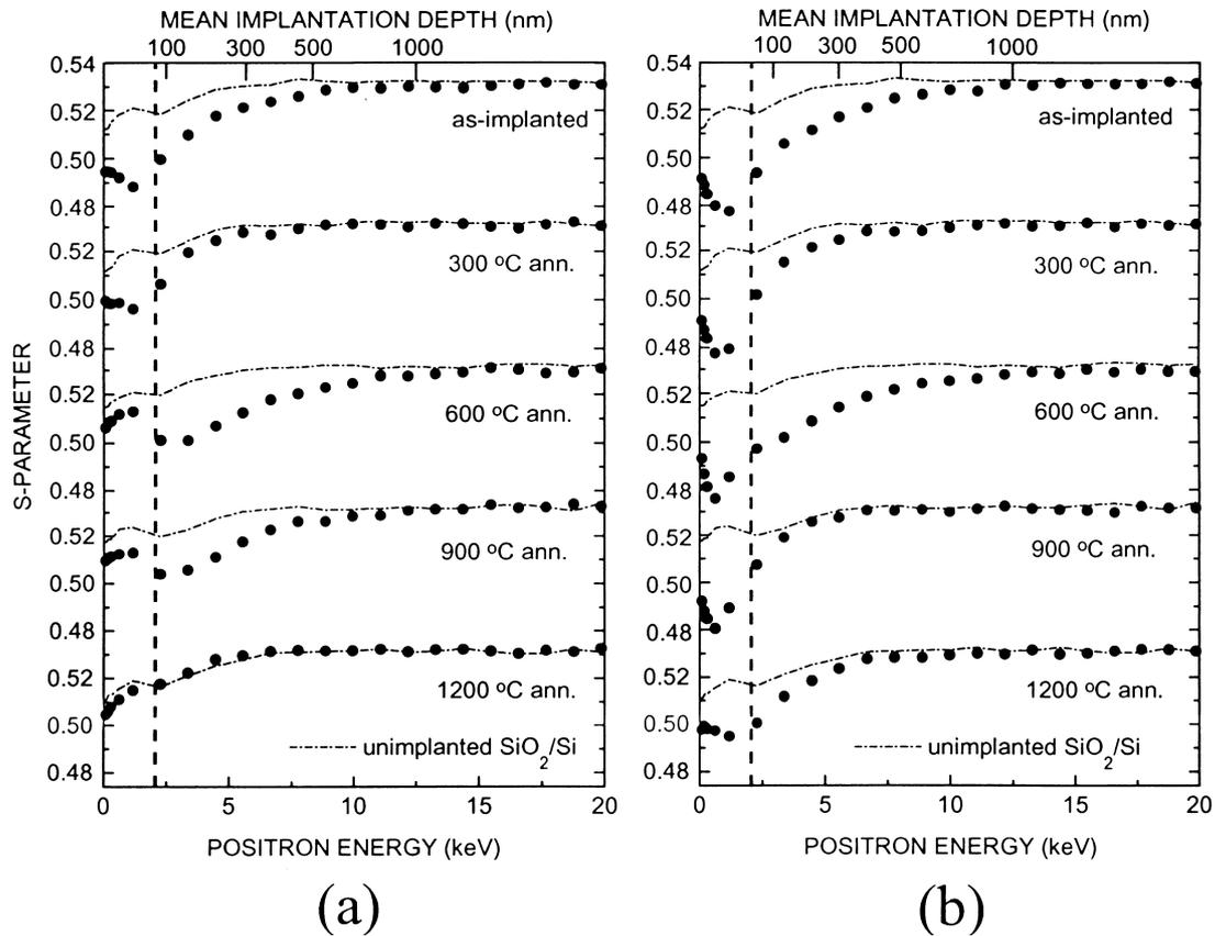
Fig. 3.  $S$ - $E$  plots for unimplanted  $\text{SiO}_2(500 \text{ \AA})/\text{Si}$  implanted with 30 keV Er ions at doses of (a)  $3.0 \times 10^{14} \text{ Er/cm}^2$  and (b)  $1.5 \times 10^{15} \text{ Er/cm}^2$  obtained after annealing. Chained lines show the  $S$ - $E$  curves for the unimplanted specimen. Dashed lines show the position of the  $\text{SiO}_2$ -Si interface.
