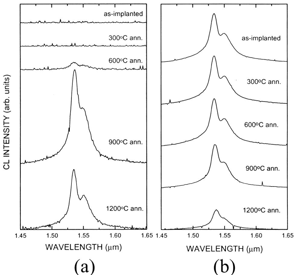
Fig. 1. Cathodoluminescence spectra at room temperature from (a) SiO<sub>2</sub>(500 Å)/Si implanted with 30 keV Er ions and (b) SiO<sub>2</sub>(5000 Å)/Si implanted 300 keV Er ions at a dose of  $1.5 \times 10^{15}$  Er/cm<sup>2</sup> recorded after each annealing.
