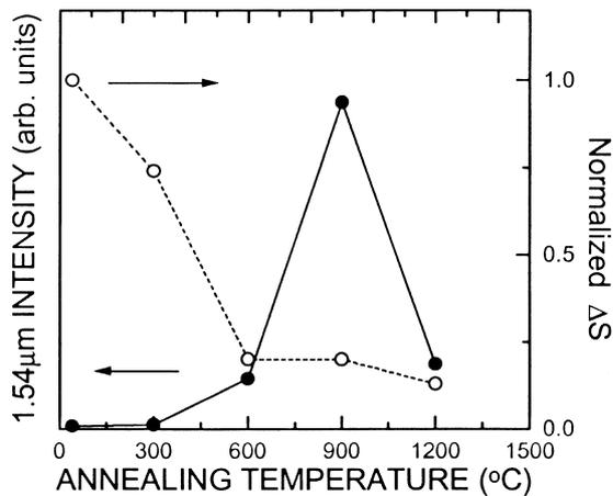
Fig. 4. Change in the  $S$ -parameter ( $\Delta S$ ) for the  $\text{SiO}_2(500 \text{ \AA})/\text{Si}$  implanted with 30 keV Er ions at a dose of  $3.0 \times 10^{14} \text{ Er/cm}^2$  from that for unimplanted  $\text{SiO}_2(500 \text{ \AA})/\text{Si}$  at  $E = 1 \text{ keV}$  and the  $1.54 \mu\text{m}$  peak intensity as a function of annealing temperature. The  $\Delta S$  is normalized to the value before annealing.
