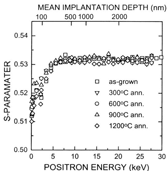
Fig. 2.  $S$ - $E$  plots for unimplanted SiO<sub>2</sub>(500 Å)/Si specimen taken after each annealing. Dashed line shows the position of the SiO<sub>2</sub>-Si interface.
