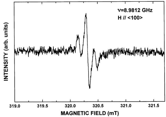
Fig. 2. ESR spectrum recorded at 296 K for the specimen irradiated with 1-MeV electrons at a fluence of  $1.1 \times 10^{18} \text{ e}^-/\text{cm}^2$ . The magnetic field was applied parallel to the  $\langle 100 \rangle$  axis
