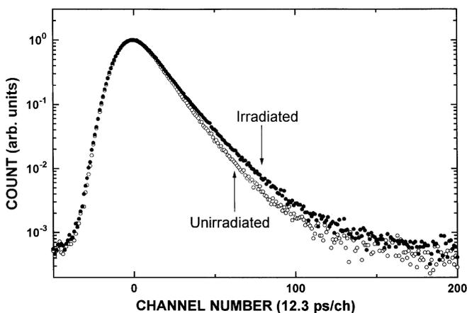
Fig. 1. Positron lifetime spectra for the unirradiated specimen (open circle) and the specimen irradiated with 1-MeV electrons at a fluence of  $1.1 \times 10^{18} \text{ e}^-/\text{cm}^2$  (filled circle)
