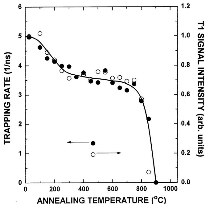
Fig. 4. Positron trapping rate responsible for the second lifetime component in Fig. 2 (filled circle) and  $T1$ -signal intensity (open circle) as a function of annealing temperature
