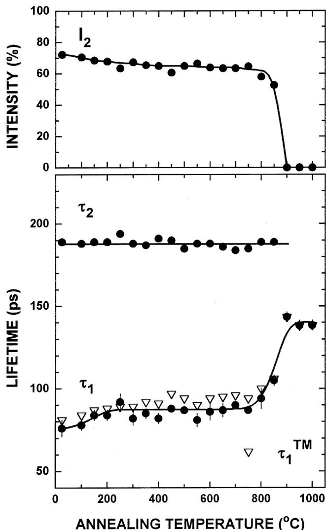
Fig. 3. Positron lifetimes ( $\tau_1$  and  $\tau_2$ ) and intensity  $I_2$  as a function of annealing temperature for the specimen irradiated with 1-MeV electrons at a fluence of  $1.1 \times 10^{18} \text{ e}^-/\text{cm}^2$ . The lifetime  $\tau_1^{\text{TM}}$  denotes the lifetime  $\tau_1$  expected from the two-state trapping model
