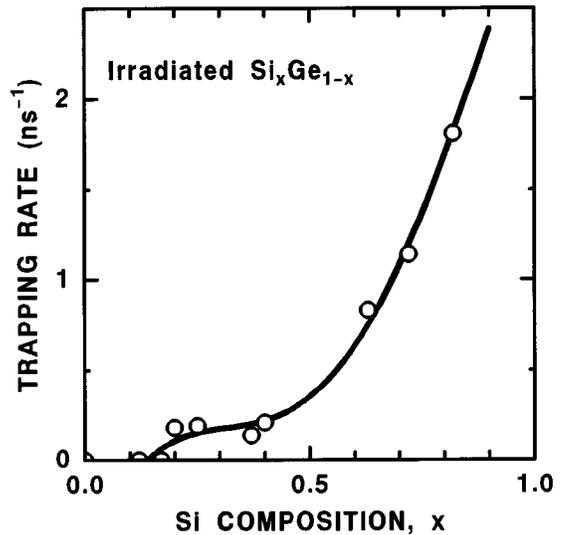
FIG. 3. Positron trapping rate due to the vacancy-type defects represented by the lifetime  $\tau_2$  in Fig. 2 as a function of the Si composition  $x$ .
