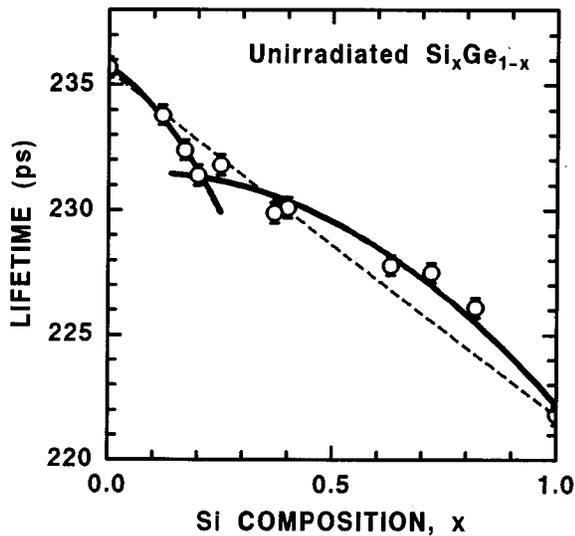
FIG. 1. Positron lifetime observed for unirradiated  $\text{Si}_x\text{Ge}_{1-x}$  crystals as a function of the Si composition  $x$ . The broken line shows the bulk lifetime expected from Vegard's law. The solid lines are the guides for eye.
