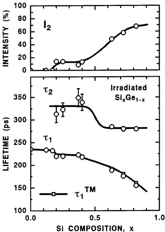
FIG. 2. Positron lifetimes ( $\tau_1$  and  $\tau_2$ ) and intensity ( $I_2$ ) observed for electron-irradiated  $\text{Si}_x\text{Ge}_{1-x}$  crystals as a function of the Si composition  $x$ . The lifetime  $\tau_1^{\text{TM}}$  denotes the  $\tau_1$  value expected from the trapping model.
