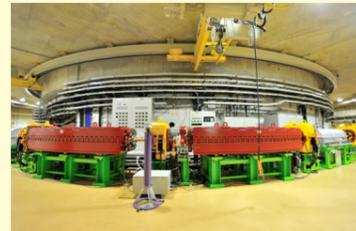
④ Bending Magnet of Synchrotron
