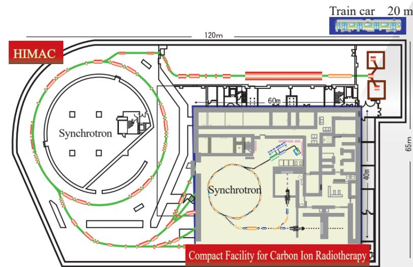
Since HIMAC was constructed for research, it has a scale of football court. The compact facility for carbon ion radiotherapy is one-third the scale and cost of HIMAC through the optimization of ion species and energy. They are at work at Gunma University, in Saga Prefecture, in Kanagawa Prefecture, in Osaka Prefecture, and at Yamagata University.
