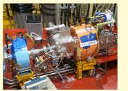
(1) ECR Ion Source This type of ion source produces highly charged carbon ions.
