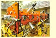
(2) RFQ Linac Linear accelerator for low-speed ions. Length: 7.3 m /up to 4% of the speed of light
