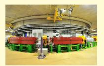
(4) Bending Magnet of Synchrotron
