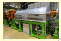
(5) RF Cavity By gradually increasing the radiofrequency, the ions are accelerated up to 84% of the speed of light.
