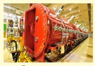
(3) Alvarez Linac Linear accelerator for mediumspeed ions. Length:24 m/up to 11% of the speed of light
