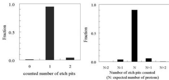
Fig 23. Counting accuracy of the single particle irradiation system measured by CR-39 detector at the cases of preset value (number of protons to be irradiated)  $N=1$  and arbitrary number  $N$  ( $N>1$ ). At  $N=1$ ,  $95.1 \pm 4.9\%$  and  $8.1\%$ , and At  $N>1$   $90.1 \pm 5.1\%$ .
