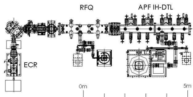
Fig 14. A schematic drawing of the compact injector. The total length of the linac cascade was 6 m.
