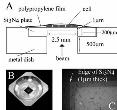
Fig 24. A is a diagram of a cell dish especially designed for SPICE and B is a photograph of the cell dish. B shows the boundary of  $200\ \mu\text{m}$  and a  $1\ \mu\text{m}$  thick portion of the  $\text{Si}_3\text{N}_4$  plate. The upper left edge is defined as the datum point
