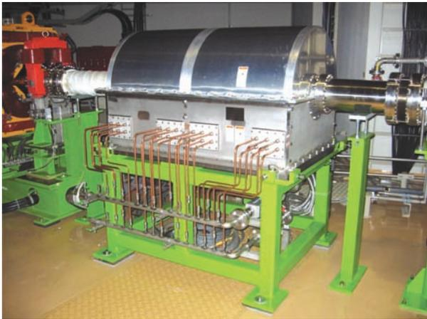
Fig 15. Acceleration cavity installed in the HIMAC synchrotron.
