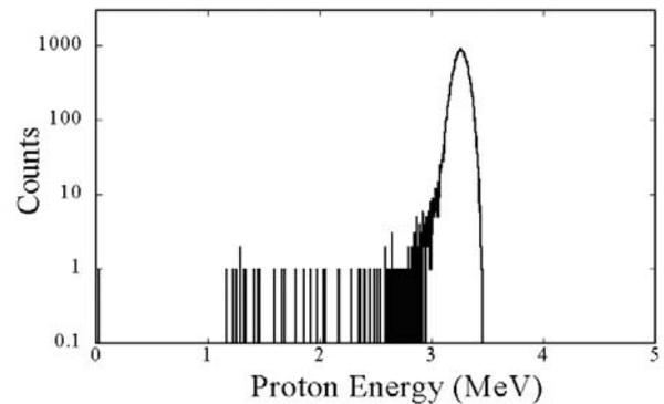
Fig 22. Typical example for the energy spectrum of the proton microbeam at the beam exit.
