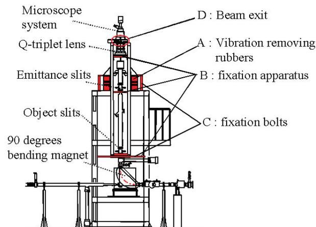
Fig 21. Schematic drawing of the SPICE beamline and its modifications. A is the vibration-removing rubber. B is the three apparatus for fixation of inner frame and the beam duct. C is the adjustable bolts to fixate the inner and outer frames.
