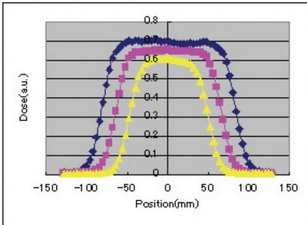
Fig 16. Dose profile of the irradiation field. The field sizes of 80, 130, 180 mm in diameter are plotted with yellow, red and blue, respectively.
