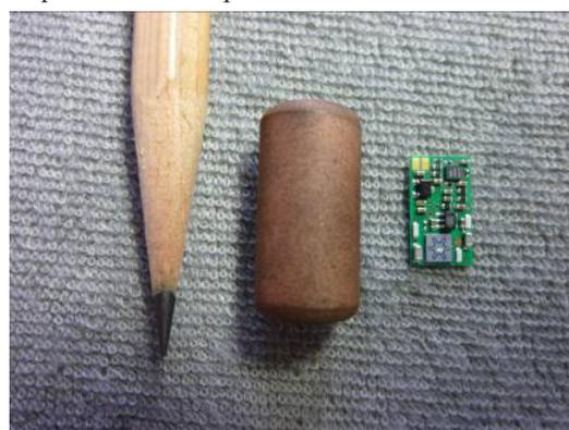
Fig.5.2. The phantom insertion type semi-conductor detector
