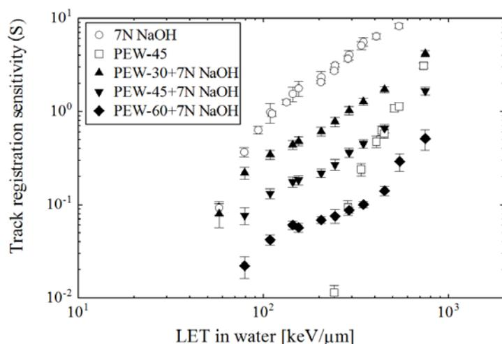
Fig.6.4. Variation of detector responses for the two-step etching method, single etching of 7N NaOH solution, and PEW-45 etching solution as a function of LET. The responses smoothly shifted to higher LET region as the ethanol concentration is increased in the PEW etching solution.
