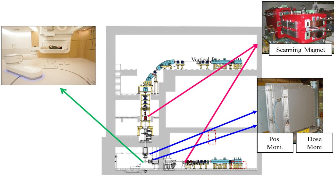
Fig. 2.5. Layout of the treatment room E.
