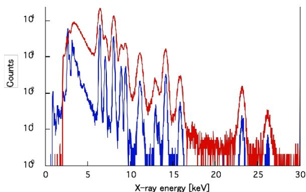
Fig.6.2 Comparison of detection efficiency by PIXE analysis of a multi-element standard sample with the existing Si(Li) detector and the new CdTe detector.
