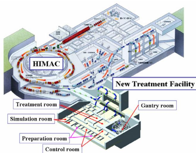
Fig. 2.4. Schematic view of the HIMAC and the new treatment research facility.
