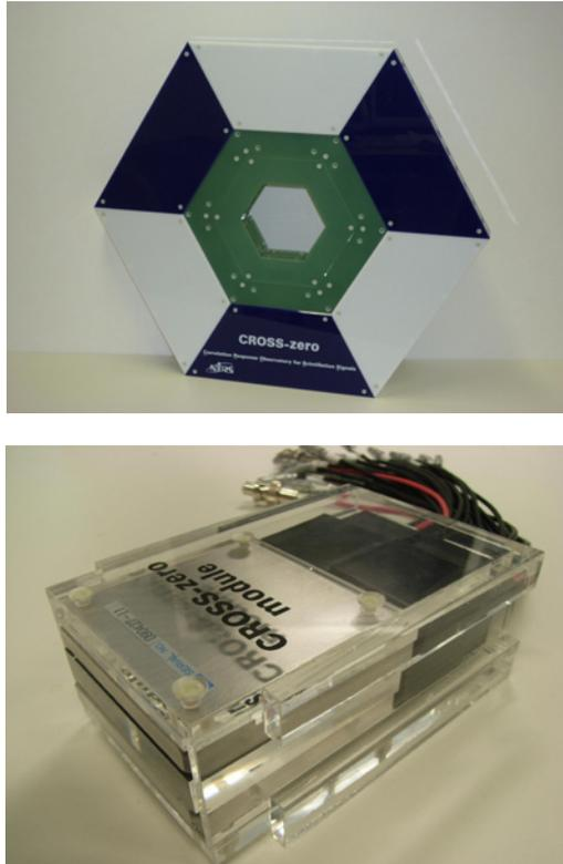
Fig. 6.5 CROSS-zero detector (top), which consists of 6 modules. Mounted in each module are an organic material, two thin rectangular NaI(Tl) scintillators, and two photomultiplier tubes (R8900, Hamamatsu Photonics K. K., Japan) (bottom).
