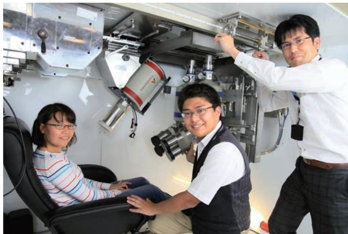
ciency of a system consisting of four Hyper-Pure Ge (HPGe) semiconductor detectors placed over the head by means of numerical simulations coupled to the adult male-reference voxel phantom developed by the International Commission on Radiological Protection (ICRP) (Fig.1) [4]. In the simulations, pulse height spectra of the HPGe detectors were calculated by tracking all physical interaction processes for a large number ( $\sim 10^7$ ) of photons from the actinides in the skull.
