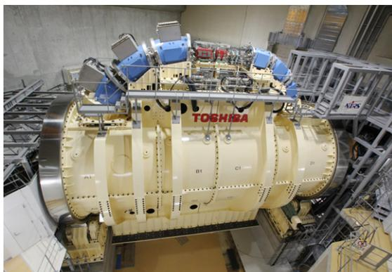
Fig.3 A photo of the superconducting rotating gantry. The superconducting and scanning magnets are colored blue and red, respectively.
