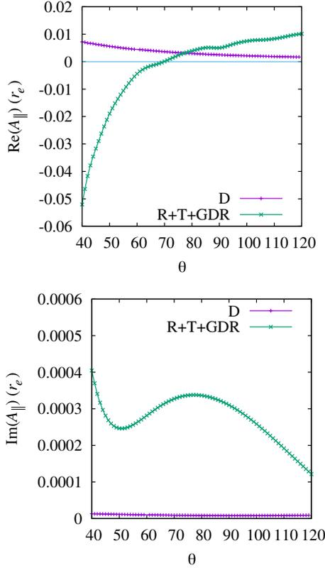
FIG. 3. The real and imaginary parts of the scattering amplitudes  $A_{\parallel}$  for  $D$  and  $R + T + GDR$  as indicated in the figures at 1100 keV of tin in units of  $r_e$ . The angular resolution is  $\Delta\theta = 1^\circ$  (excluding  $60^\circ$ ) with a relative error of 1% for  $D$ .
