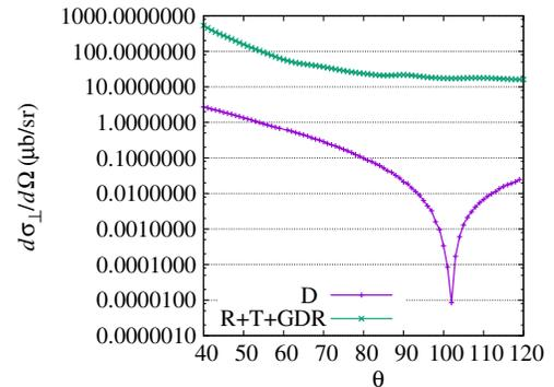
FIG. 5. The differential scattering amplitude  $d\sigma_{\perp}/d\Omega$  for  $D$  and  $R + T + GDR$  as indicated in the figure for tin at 1.1 MeV. The angular resolution is  $\Delta\theta = 1^\circ$  (excluding  $60^\circ$ ) with a relative error of 1% for  $D$ .
