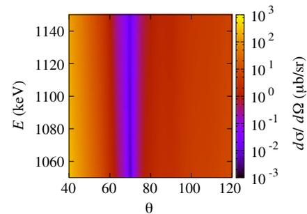
FIG. 2. The differential cross section  $d\sigma_{\parallel R+T+GDR}/d\Omega$  for tin including  $R + T + GDR$  for scattering angles from  $40^\circ \leq \theta \leq 120^\circ$  in the scattering plane. The angular resolution is  $\Delta\theta = 0.15^\circ$ , and the energy resolution is 1 eV.
