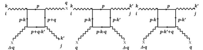
FIG. 1. Delbrück scattering represented by lowest-order Feynman diagrams.  $k$  and  $k'$  are the 4-vector momenta of the incoming and outgoing photons, respectively, and  $i$  and  $j$  are their polarization directions, respectively.  $\Delta = k' - k$  is the momentum transfer. The  $X$  represents the Coulomb field of the nucleus in which  $q$  is the field momentum.
