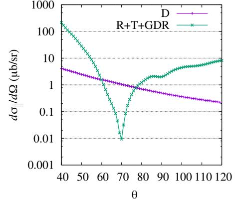
FIG. 4. The differential scattering amplitude  $d\sigma_{\parallel}/d\Omega$  for  $D$  and  $R + T + GDR$  as indicated in the figure for tin at 1100 keV. The angular resolution is  $\Delta\theta = 1^\circ$  (excluding  $60^\circ$ ) with a relative error of 1% for  $D$ .
