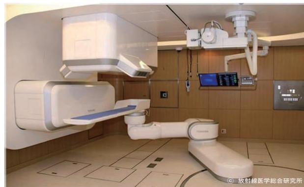
Fig.3 Treatment Room E with two fixed beam ports and SCARA-type robotic arm.
