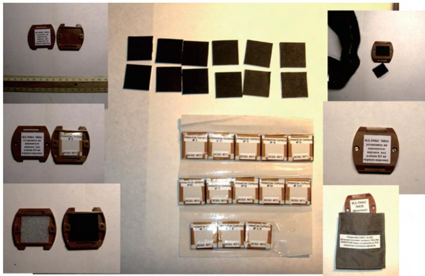
Fig.2 Passive detectors of NIRS and IBMP, Russia, for the protective curtain project.
