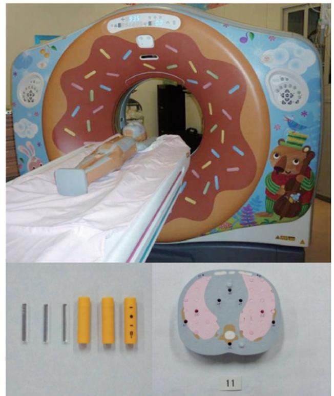
Fig.3 Organ dose measurements using anthropomorphic phantoms and glass dosimeters
