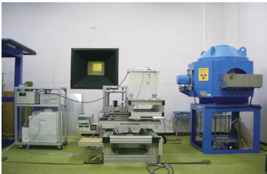
Fig. 1 NIRS  $^{60}\text{Co}$  gamma-ray standard field for  $N_{D,w}$  calibration of therapy-level dosimeter
