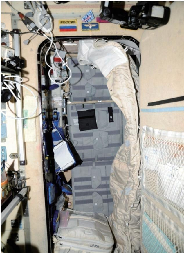
Fig.3 The protective curtains which were installed for our passive detector packages in the ISS.
