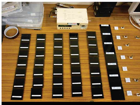
Fig. 7-6. Photograph of detector packages in the 2nd Proton-Intercomparison experiments.
