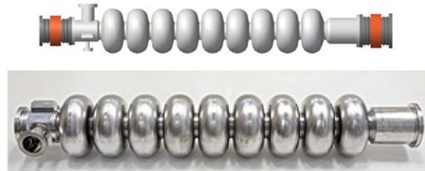
Figure 27. ERL cavity developed by KEK/JAEA/U-Tokyo. The cavity has a 9-cell shape and is operated at 1.3 GHz [104].
