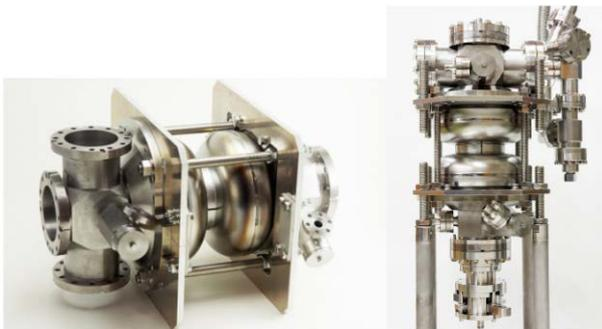
Figure 26. Injector cavity developed at KEK. The cavity has a 2-cell shape and is operated at 1.3 GHz. Five HOM couplers are installed at both sides of the beam pipe [103].
