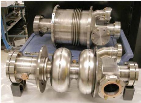
Figure 25. Injector cavity developed at Cornell University. The cavity has a 2-cell shape and is operated at 1.3 GHz [58].
