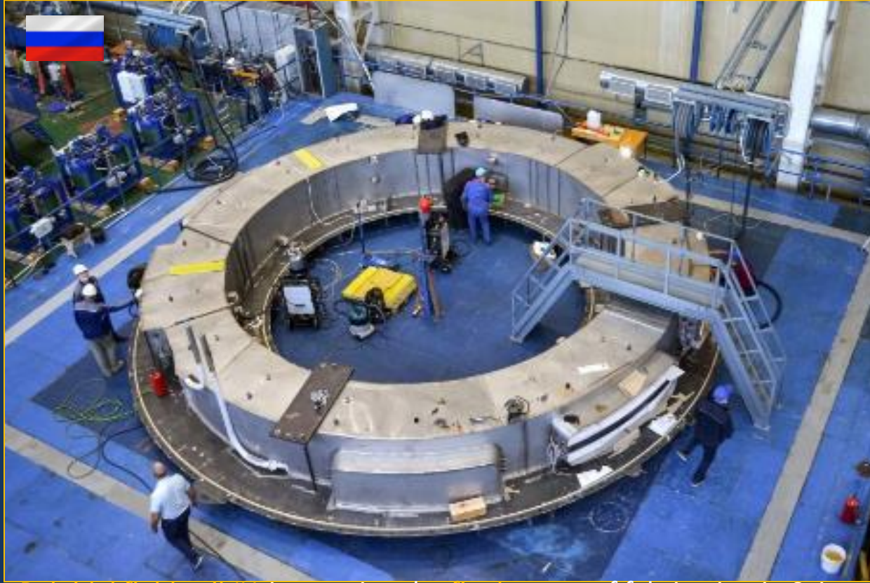
Poloidal field coil #1 is entering the final stages of fabrication in Saint-Petersburg.
