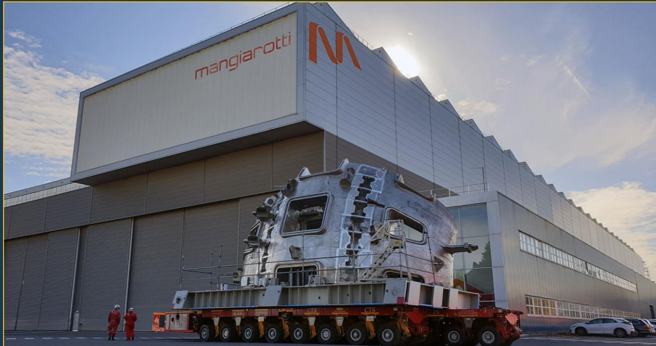
Five vacuum vessel sectors are under fabrication in Italy. Completion rates range from 76 to 97%
