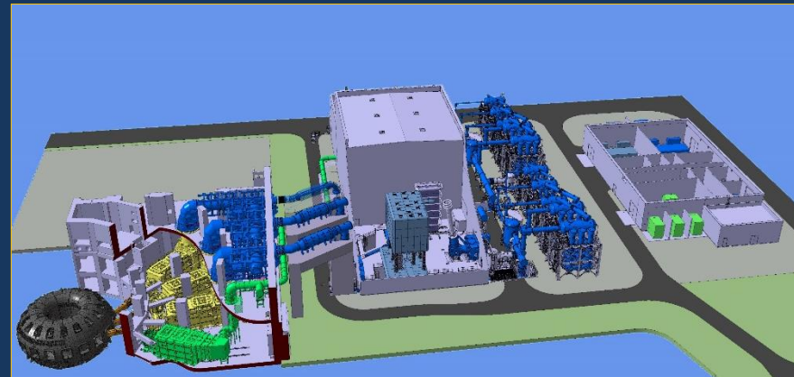
Neutral beam power supply bdg. 1 MeV voltage fed to the NB injectors
