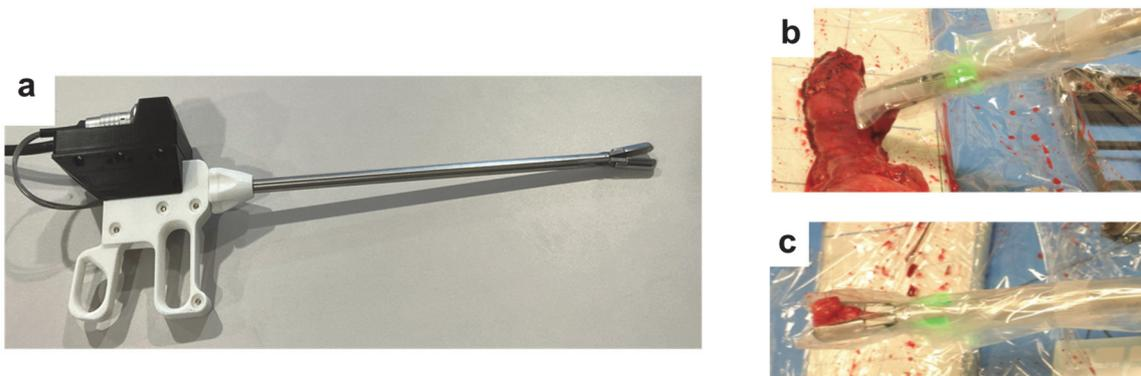
**Figure 2** Forceps-type PET (a), LNs measurement with forceps-type PET used in an operating room (b,c).
