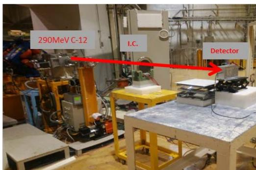
Figure 5 Experimental setup of the evaluation of the rubrene single crystal in HIMAC.
