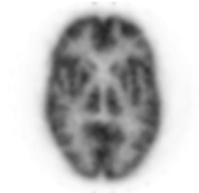
**Figure 5** PET image of the hemispherical Hoffman phantom obtained by the helmet-neck PET prototype.
