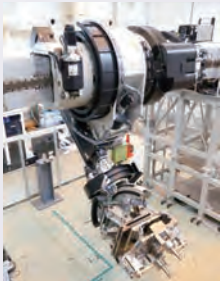
Robotic arm for fusion reactor maintenance and inspection
