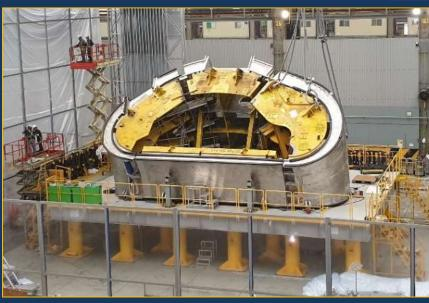
4 out of 9 sectors for the vacuum vessel are being manufactured by Hyunday Heavy Industries. The first one is now completed.
