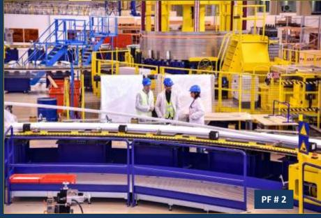
Too large to be transported by road, four of ITER's six ring-shaped magnets (the poloidal field coils, 17 to 24 m, in diametre) will be assembled on site by Europe in this 12,000 m² facility. Resin impregnation ongoing for PF Coil # 5 (17 m. diametre, ~ 350 tonnes) and work has started on PF Coil # 2 (17 m. diametre, 204 tonnes)
