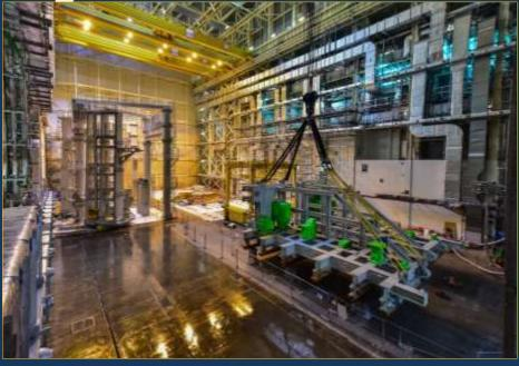
Manufactured in Korea, two sub-assembly tools (SSAT-1 & 2) will handle loads of up to 1,500 tonnes. Functional tests under load are complete. The floor of the 6,000 m2, 60-metre high Assembly Hall is being coated with epoxy resin to ensure cleanliness during assembly operations. The two halves of the upending tool were delivered last week.
