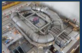
Cold tests are finalized at Mitsubishi Electric Corporation for the first winding pack of TF coil # 12
