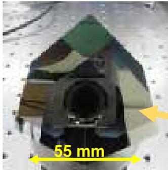
Retroreflector made by grinding tungsten material
