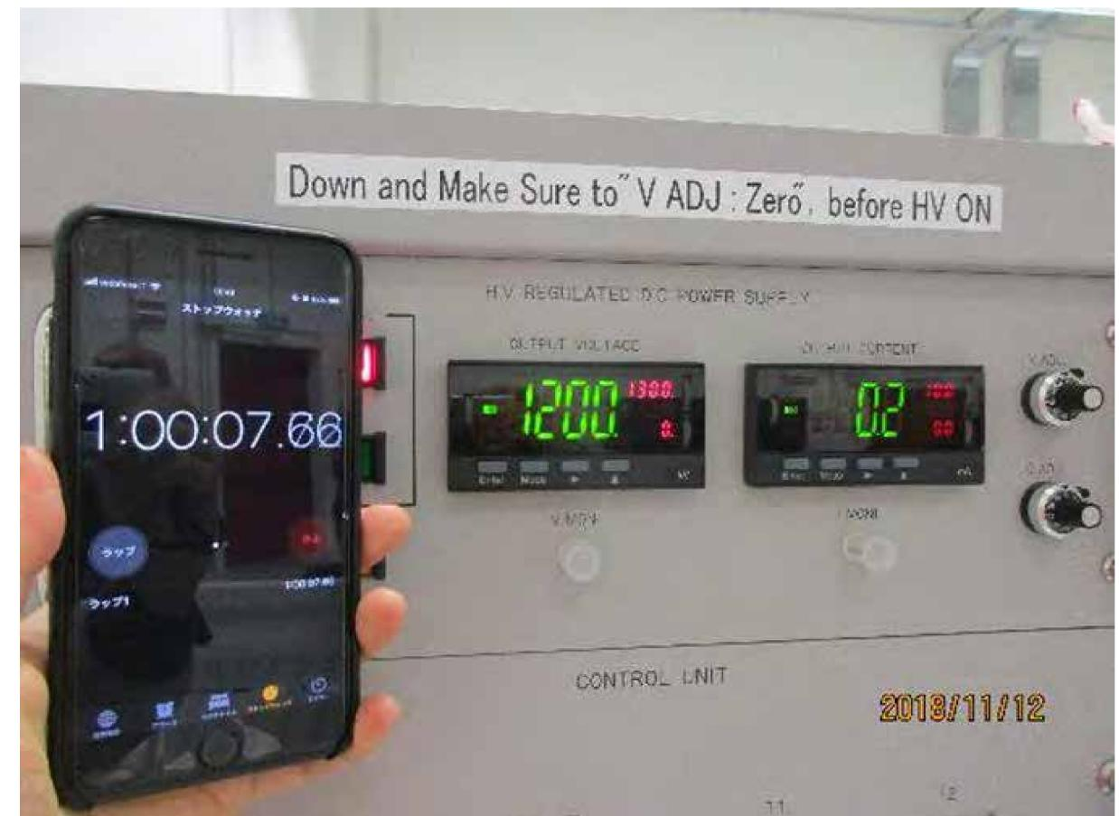
Photo of 2<sup>nd</sup> withstand voltage test
