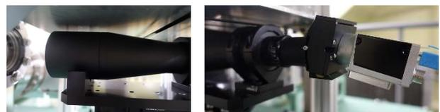
Fig. 2 Telecentric lens (left) and camera tilt unit (right)
