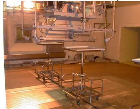
Electron irradiation room with conveyor system
