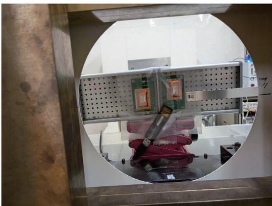
Figure 2. Si-detectors at test positions of the HIMAC BIO exposure room.
