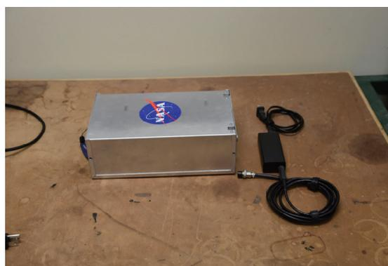
Figure 1. (t) Block diagram of the AirTED instrument. (b) Photo of the AirTED detector for use aboard high altitude aircraft.
