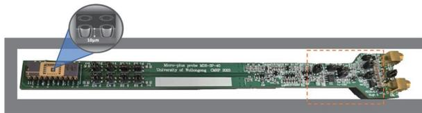
Fig. 2: MicroPlus2 Probe with SOI microdosimeter inserted. Built-in shaping amplifier indicated in orange region.
