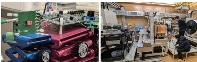
Fig. 2: Setup of the beam test in 2024. Left) The CIGS detector Right) Whole view at the biological irradiation room.
