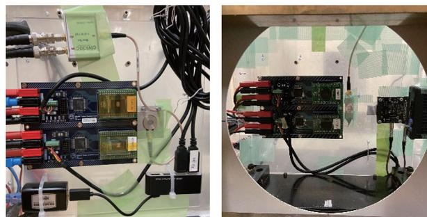
Fig. 1 SRAM and diode setup irradiated at HIMAC in 2024 (left) and 2025 (right).
