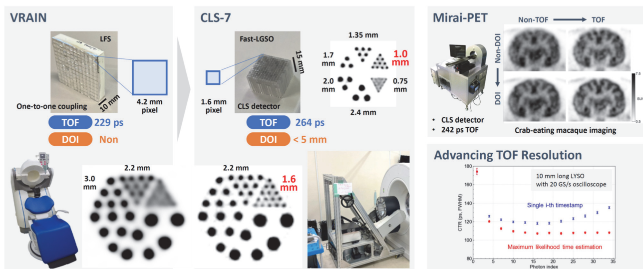
Figure 3 The high spatial resolution of 2.2 mm achieved by VRAIN (left) is surpassed by the crosshair light-sharing (CLS) detector, which combines time-of-flight (TOF) and depth-of-interaction (DOI) measurement capabilities with a finer scintillator pitch. The developed prototype (CLS-7) demonstrated 1 mm resolution, approaching the theoretical limit for brain PET (middle). The CLS detector has already been implemented in a small-animal PET scanner, Mirai-PET, demonstrating the effectiveness of TOF and DOI measurements even in monkey brain imaging (upper right). Further improvement in TOF resolution is expected, for example, by resolving scintillation light into individual photons (lower right).
