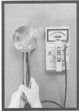
Photo. 2.1.2-1 Measurement to estimate conversion coefficient.
