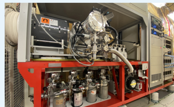
Multi-ion source for more advanced treatment
