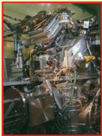
High heat flux testing of the test blanket module and divertor.
