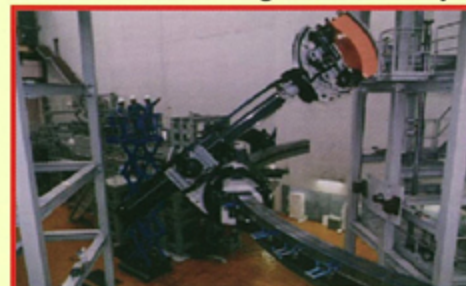
Testing of remote handling equipment
