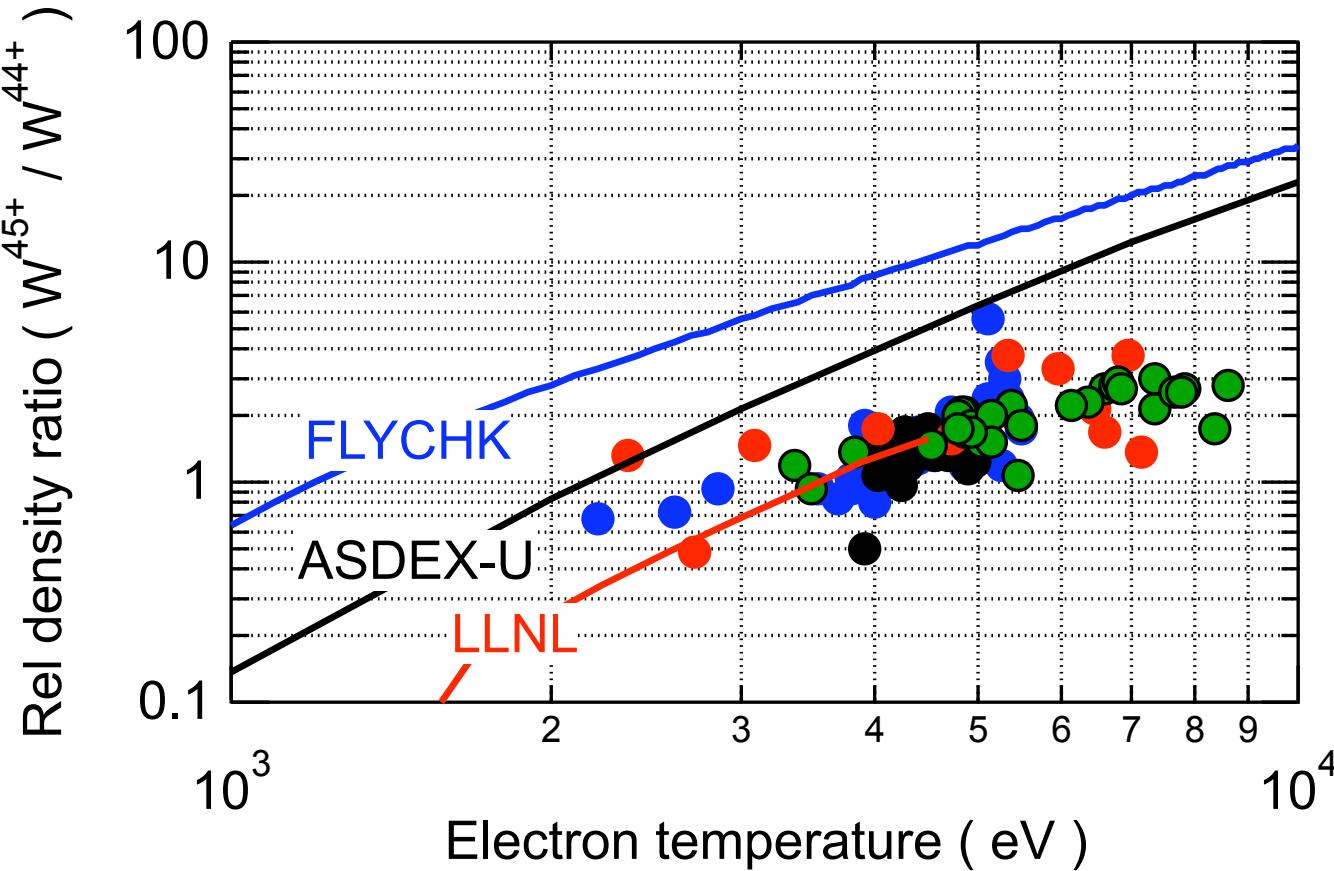
At high temperature, blend of  $W^{44+}$  with  $W^{43+}, 42+$  should be low
