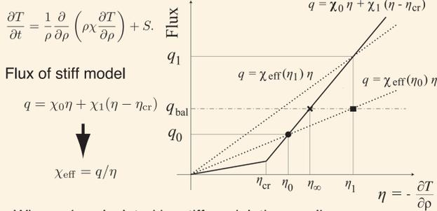
When  $\chi$  is calculated by stiff model, the non-linear iteration does not converge for large time steps. Then the size of time step must be very small for stable calculation.
