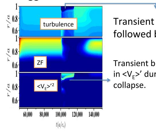
Transient collapse of turbulence, followed by return to L-mode
