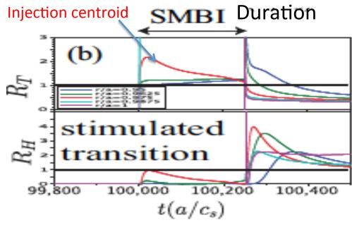
Stimulated transition:  $R_T$ (edge) and  $R_H$  peak simultaneously, at transition.
